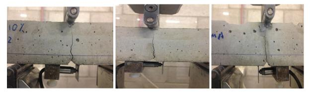
Figure 1: Mortar samples containing one capsule from PLA+10% impact modifier (left), PLA (middle) and PMMA (right) after three-point-bending test (crack width:0.9 mm)
